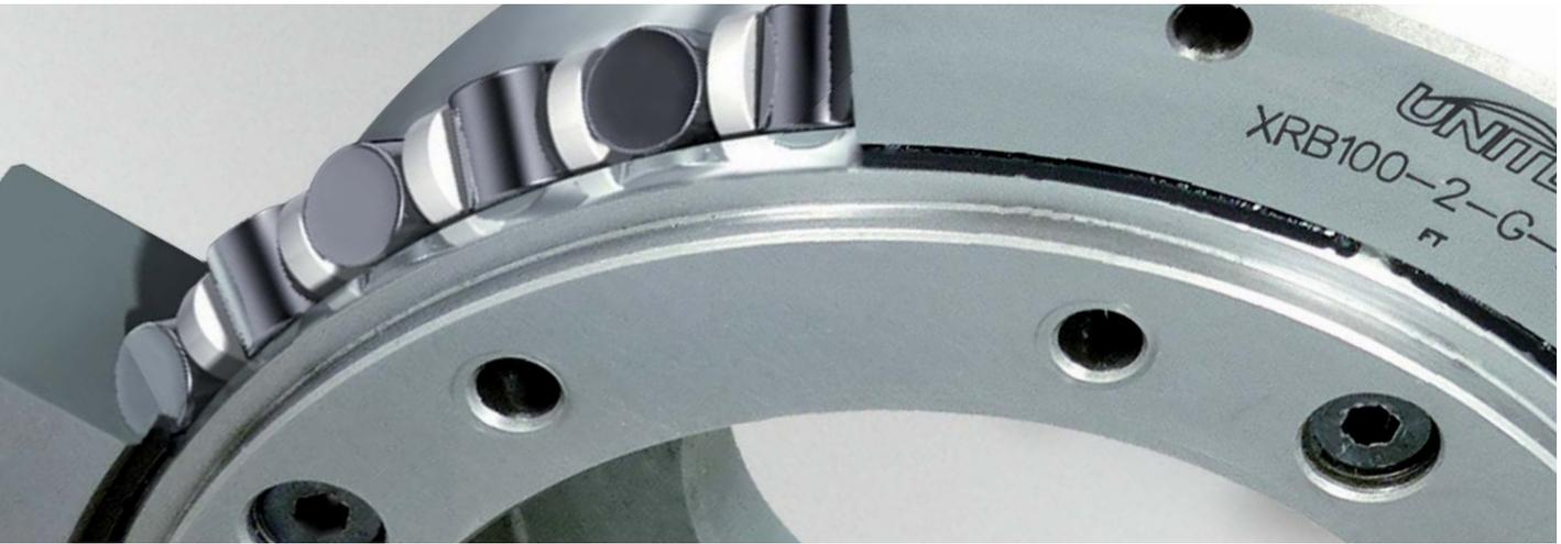
This type of bearings is mainly used into the industrial branches of the machine tools, general automation, medical machineries, defense industry and for all those applications which require an extremely compact design together with high stiffness and accuracy requirements. All the UNITEC cross roller bearing executions can be supplied from min. bore 40 mm up to outer diameter of 800 mm.
