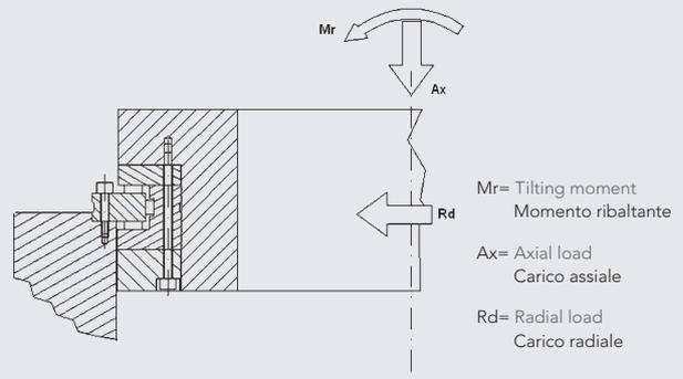
It is possible to improve the stiffness of the RTB bearing, by using a thrust washer, as shown in pic 2.2
