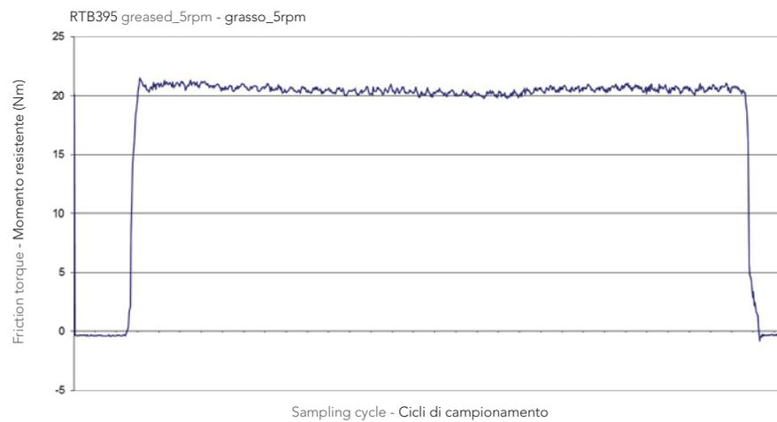
Pic 5.1 and Pic 5.2 report the rolling torque charts at 5 rpm of the RTB 395 and RTB 120. Note that the starting torque peak is negligible.
