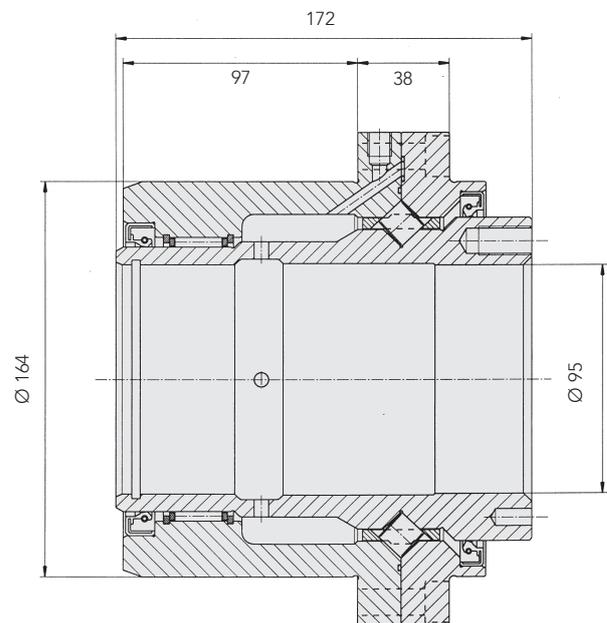
Special bearings for rotating nut support.
