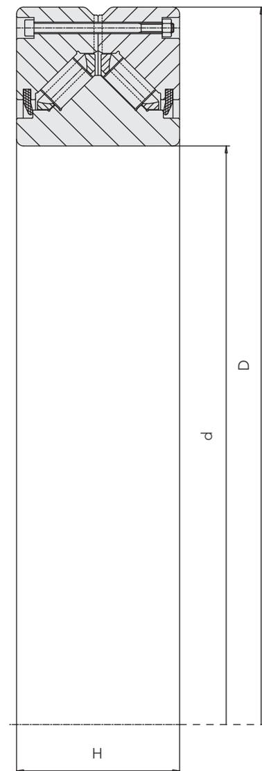
Customized double row axial/radial cylindrical roller bearing
