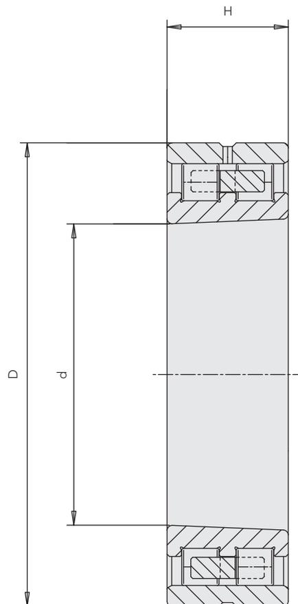
NN bearing with tapered bore - Cuscinetto NN a foro conico
