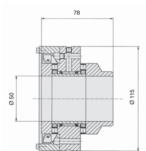
SRB special with integrated seal carrier
