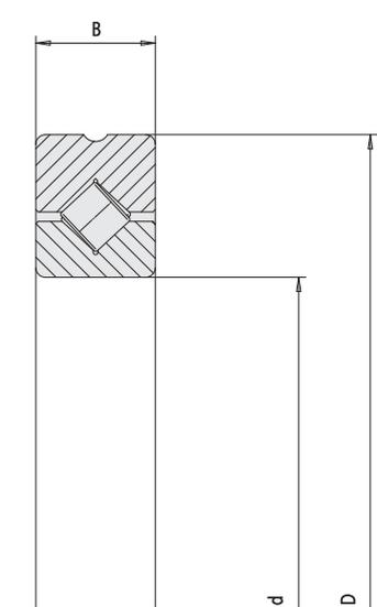
UNITEC XRB crossed roller bearings can be provided with
