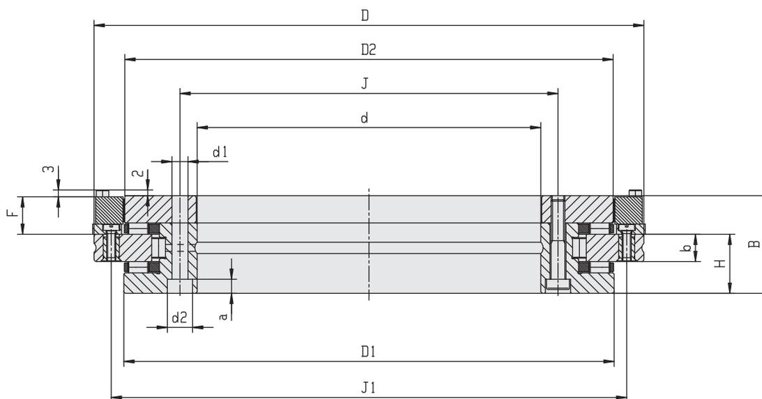
NOTE - The dimensions indicated in the table below refer to the sensor heads integration. Sizes marked with \* differ from relative standard RTB bearings, because of the increased flange thickness.
