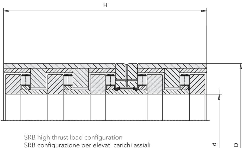
SRB high thrust load configuration
