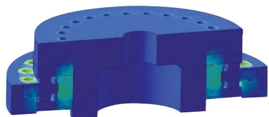
Fig. 2.4 Induced tension stresses
